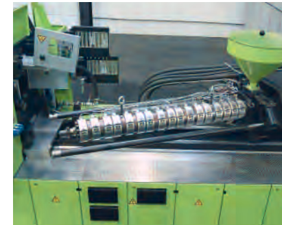
The swivelling injection unit simplifies maintenance work on the plasticizing assembly
