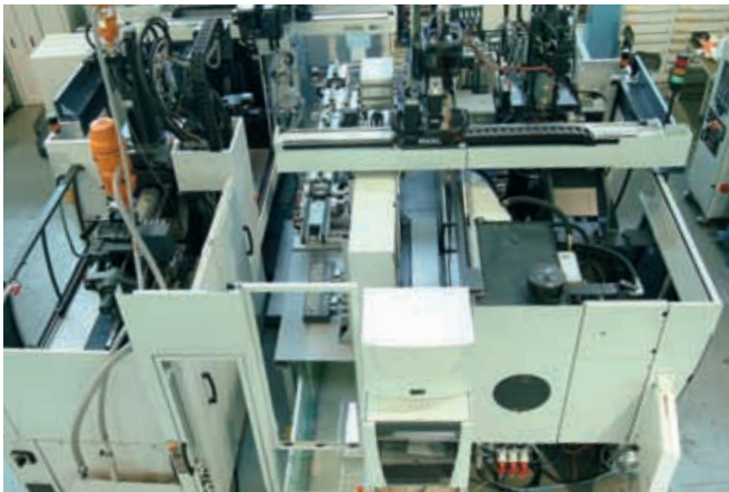
Production cell consisting of two ENGEL victory injection moulding machines each equipped with an ENGEL ERC handling robot for automatic demoulding and stacking on a joint assembly station between the machines. Photo: PARltec GmbH, Weilheim / Germany
