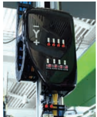
The clearly arranged display of vacuum and compressed air circuits and the simple means of switching over from vacuum to compressed air and vice versa considerably reduces the work of setting up and adjusting the robot
