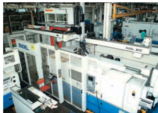
ENGEL ERC robot for the handling of workpieces on a CNC lathe
