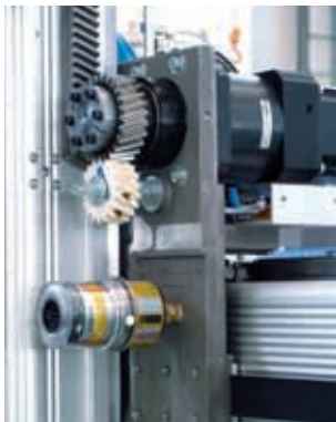
The rack-and-pinion drives are permanently lubricated for long service life and minimum maintenance
