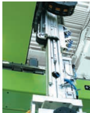
All ENGEL robots are equipped, from size ERC 63 upwards, with a telescopic vertical axis as standard, thus keeping the overall height of the machine within an acceptable limit. The double guide system ensures optimum rigidity
