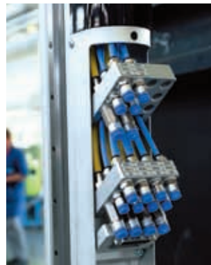
Minimum changeover times thanks to rapid-action coupling system mounted directly on the vertical axis
