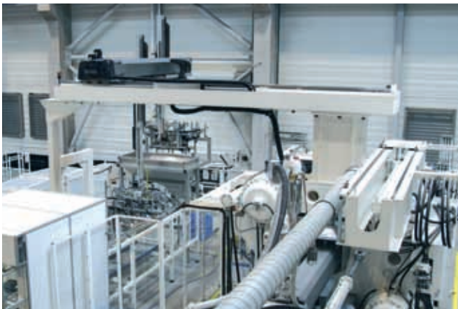
Example of a production cell based on one ENGEL duo large-capacity injection moulding machine. An ENGEL ERC 134 with two vertical axes simultaneously places inserts into the injection moulding machine, demoulds the moulded composite parts and transfers them to the downstream finishing station. Photo: Mobis Slovakia s.r.o., Zilina / Slovakia
