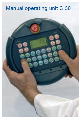
Besides the programming facility via the machine control system, the robot functions can be programmed and activated via the hand-held C30 or C100 operator terminals. This is convenient, for example, when the machine operator is working in immediate proximity to the peripherals
