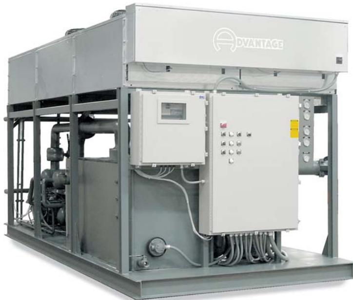
**OACS Series** chillers are designed for outdoor installations in many climates. The fully charged air-cooled refrigerant chiller, and pump tank station are packaged in a single frame that minimizes costly field installation.
