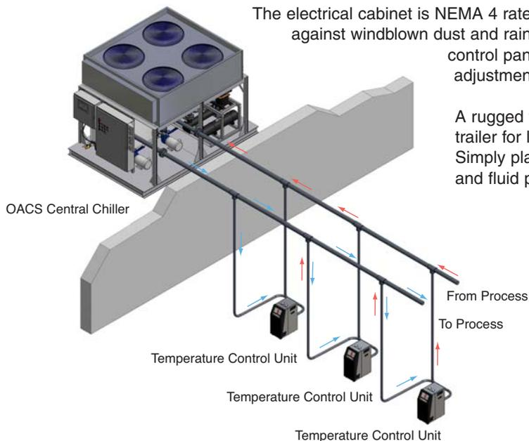
The electrical cabinet is NEMA 4 rated which means it is designed for outdoor use to provide protection against windblown dust and rain. The control instrument is visible through a viewing window in the control panel so that the chiller status can be easily monitored and adjustments can be made.
