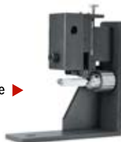
Step 3: Rotate the product to attain multiple points of measurement as well as concentricity and ovality Concentricity = \Delta (A - B) Ovality = \Delta C
